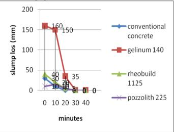
This is the graph showing combination of three superplasticizer and conventional concrete showing there slump loss at every 10 min, from this graph it is shown that rehobuild1125 show maximum slump at 0min but is not workable, after 20 min its workability fall to zero. But the conventional concrete is workable for 30 min
