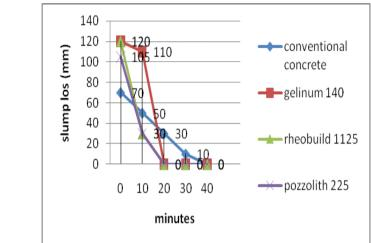
This is the graph showing combination of three super plasticizer and conventional concrete showing there slump loss at every 10 min, from this graph it is shown that Rehobuild1125 show maximum slump at 0min but is not workable, after 20 min its workability fall to zero. But the conventional concrete is workable for 30 min.
